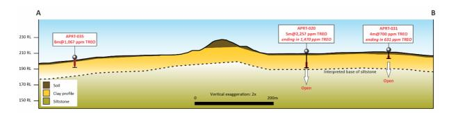
Figure 3. Representative cross-section showing high-grade REE results
