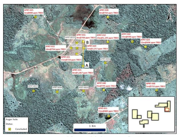
Figure 2. Apui ENE drilling. Auger holes location on satellite image
