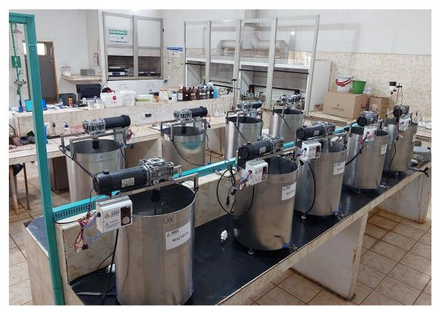
Figure 5 – Bioleach assay reactors installed in the Catalão laboratory
