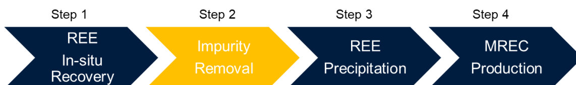
Figure 5. Step 2 of impurity removal in the simple 4 step process flow sheet to produce an MREC.
