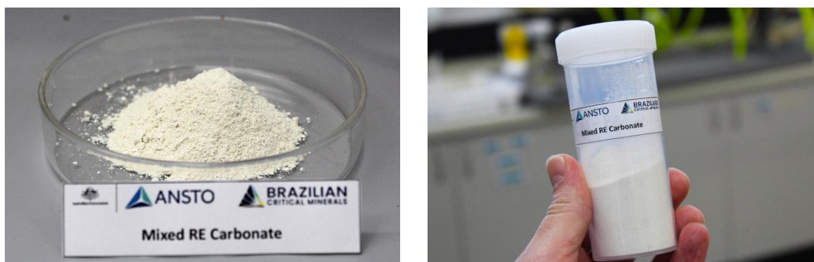
Figure 4. Final Mixed rare earth carbonate product, 33.2 grams, produced at the ANSTO facilities in Sydney.
