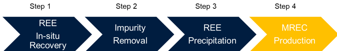
Figure 2. Simple 4 step process flow sheet for ionic clay MREC production at Ema Project
